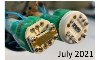
Comparison between graphene and GaAs QHRs from PTB at BIPM
