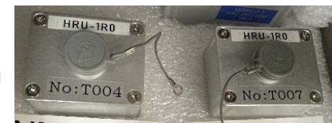
Prototypes of Alpha/NMIJ resistance standards
