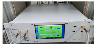
Low frequency attenuation measurement system
