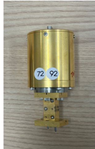
KRISS D-band direct comparison system and transfer standard
