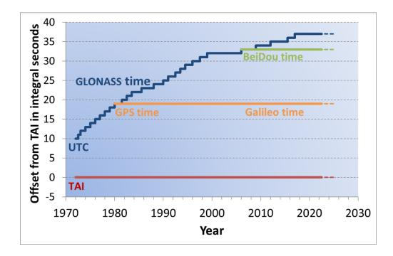
**Figure 1.** Offset between UTC, the GNSS internal time scales, and International Atomic Time TAI.
