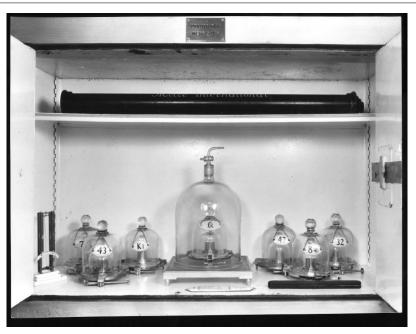
The old depository of metric prototypes. The international standard of the metre (upper part). he international prototype of the kilogram with its six witnesses.
