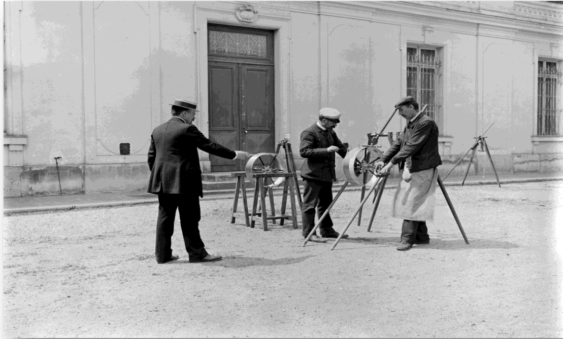
Guillaume carrying out measurements with invar threads and Jäderin's devices in the courtyard of the BIPM in 1907 (© Jacques Boyer_Roger-Viollet)
