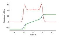
Figure 1. **A.** Sample gated using only chemical gating shows welldefined quantization at 2K. The polymer spacer thickness is such that the doping at 2K reaches  $n=2 \cdot 10^{11} \text{ cm}^{-2}$  electrons. Mobility exceeds 7000 cm<sup>2</sup>/Vs.
