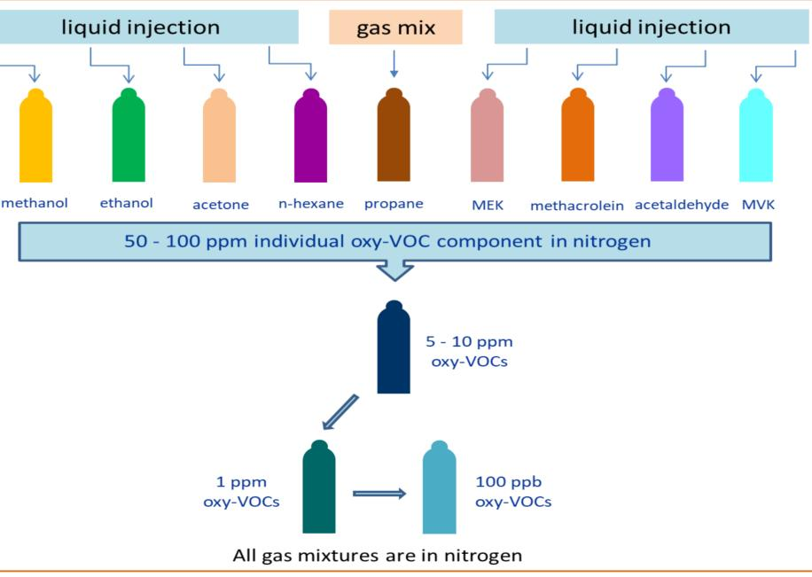
Figure 6: Preparation scheme of VSL reference gas mixtures for oxygenated VOCs. Preparation method: gravimetric according to ISO 6142-1:2015.
