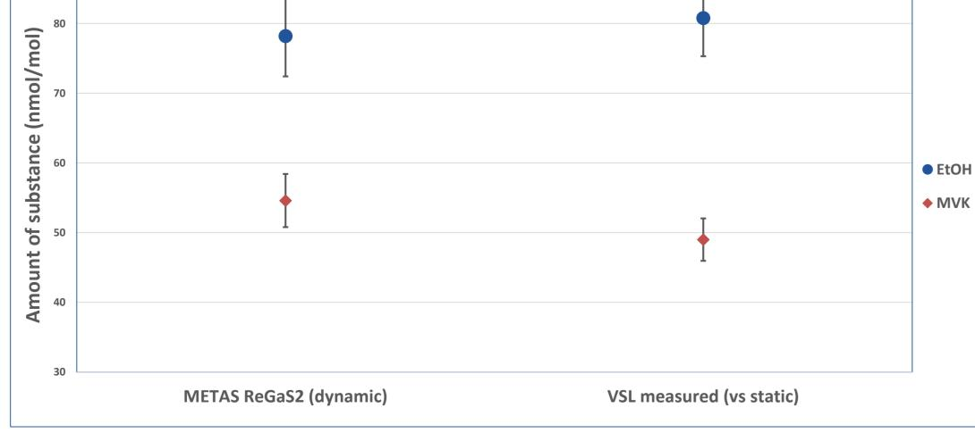
Figure 7: Comparison of Ethanol and Methyl Vinyl Ketone (MVK) produced dynamically with ReGaS2 (METAS) and gravimetrically in novel cylinders (VSL). The blue and red dots are the amount of substance fraction of Ethanol and MVK respectively. Error bars represent uncertainties (k=2)
