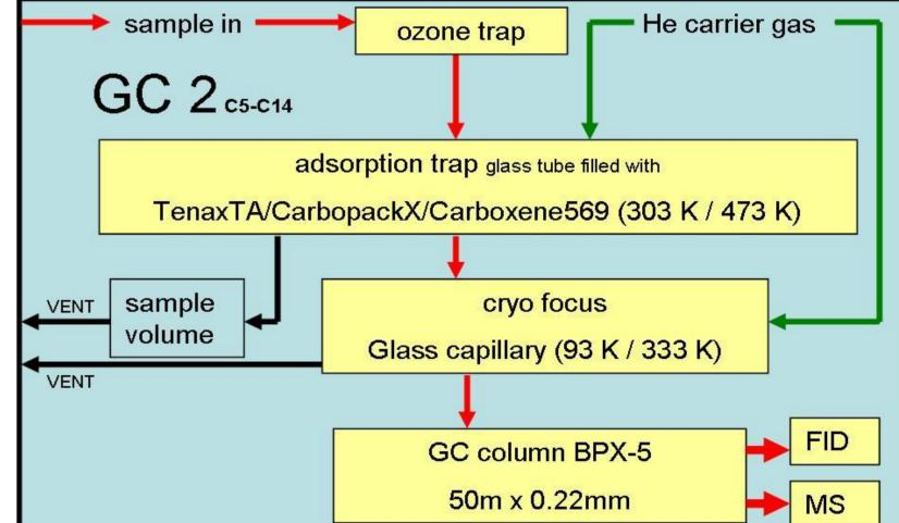
Figure 9: Schematic of the MOHp GC-FID/MS system for biogenic VOCs
