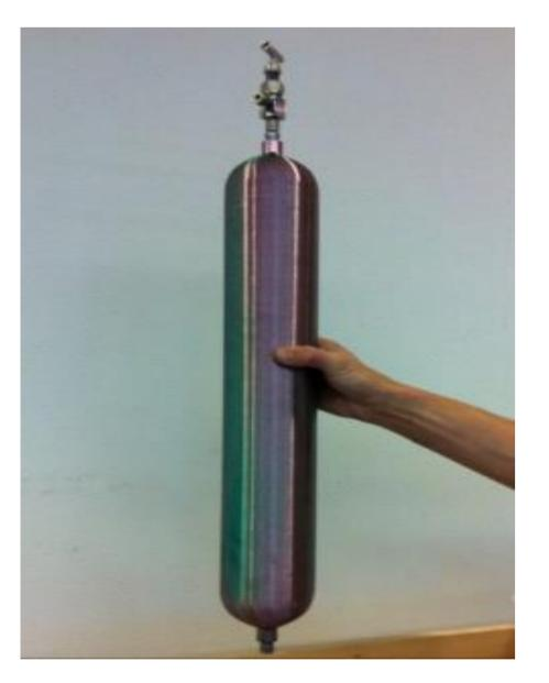
Figure 5: Picture of novel coated stainless steel cylinder used for preparation of VSL reference gas mixtures.
