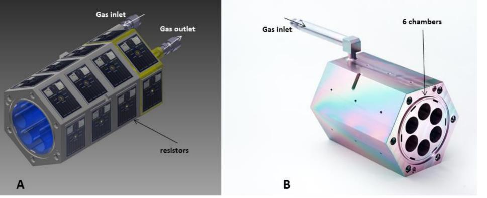
Figure 2: Computer-Aided Design (A) and picture (B) of the in-house developed oven of ReGaS2 with 6 permeation chambers. One chamber is reserved for the internal temperature sensor. The oven is entirely coated with SilcoNert<sup>®</sup>2000.
