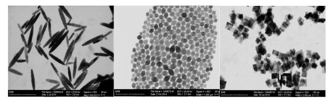
HR-SEM images of rutile, anatase and brookite TiO<sub>2</sub> nanoparticles
