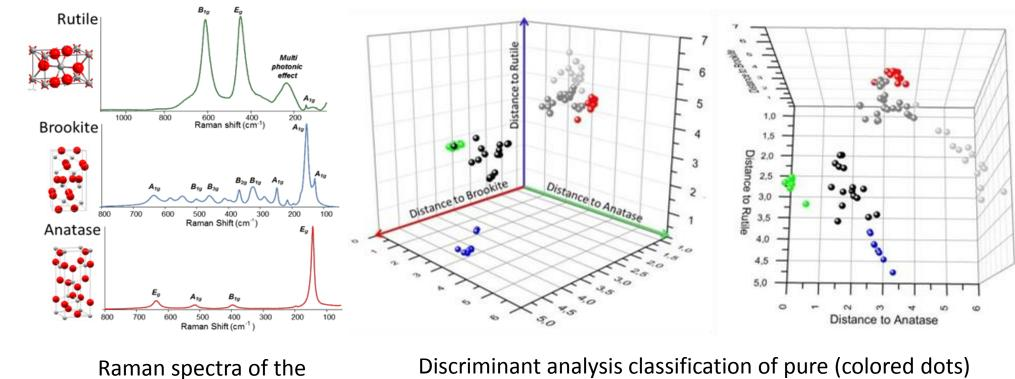
three different polymorphs an binary (grey scale dots)  $TiO_2$  mixtures
