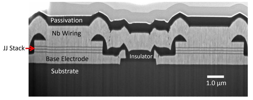
Cross-section along microwave coplanar waveguide
