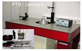
Angular vibration calibration (PTB)
