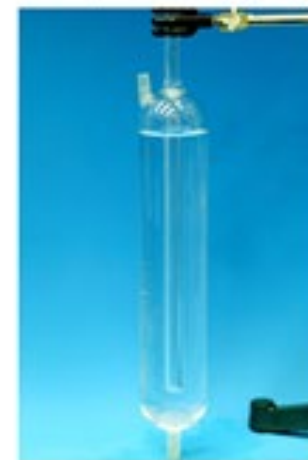
Water triple-point cell
