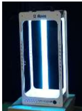
Prototype machine supplied with a UV-C PL type lamp
