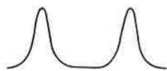
(a) VARIATION IN CENTRAL FRINGE INTENSITY WITH CHANGE IN OPTICAL PATH DIFFERENCE.
