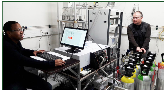
N. Ntsasa (NMISA) and P. Moussay (BIPM) measuring isotope ratios of \text{CO}_2 in air standards with FTIR
